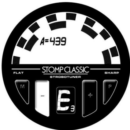
The Stomp Classic can be calibrated from A=390Hz to A=490Hz in 1Hz increments.
